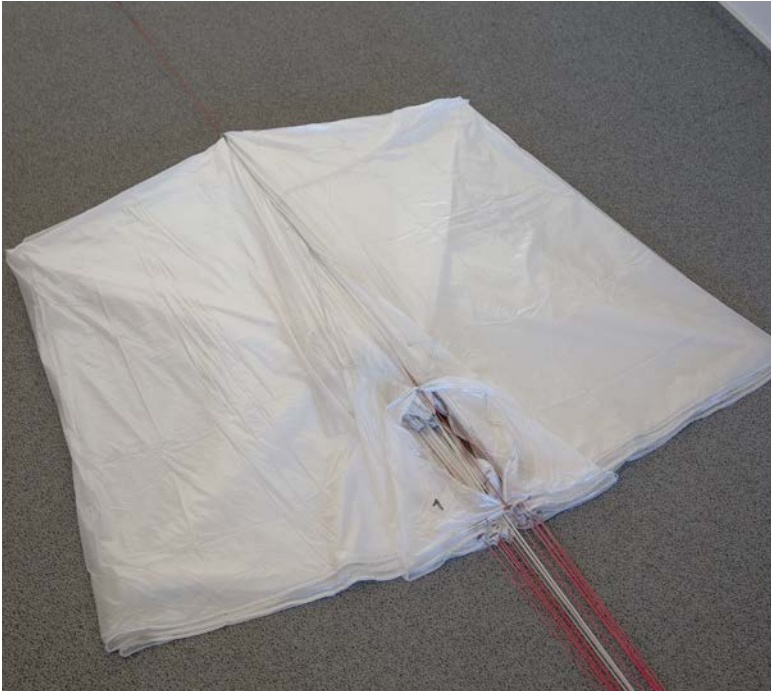
▲ The last corner is being laid out and the 1 stays on the left side
