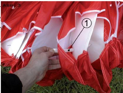
Once all reinforcements are precisely beaded and gathered up you can attach the velcro to its counterpart and the neatly stacked Mylar reinforcement will stay in shape.
