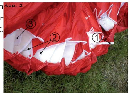
Press each reinforcement neatly onto the next. That will make for a strong packing that is protected from bending.
