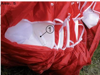
That's what the finished glider looks like. Now the back part can be folded rail by rail and rolled up.
